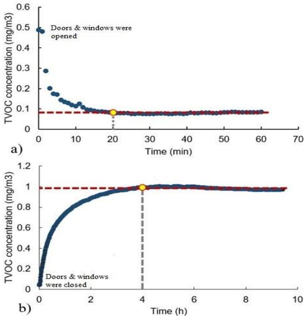
Fig.1. The variation of in-cabin TVOC concentration with time when vehicle was a) ventilated and b) closed in pre-experiment.
