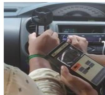
Fig.2. Measuring air flow velocity from vents.
