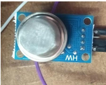
Fig. 3.MQ-138 gas sensor.
