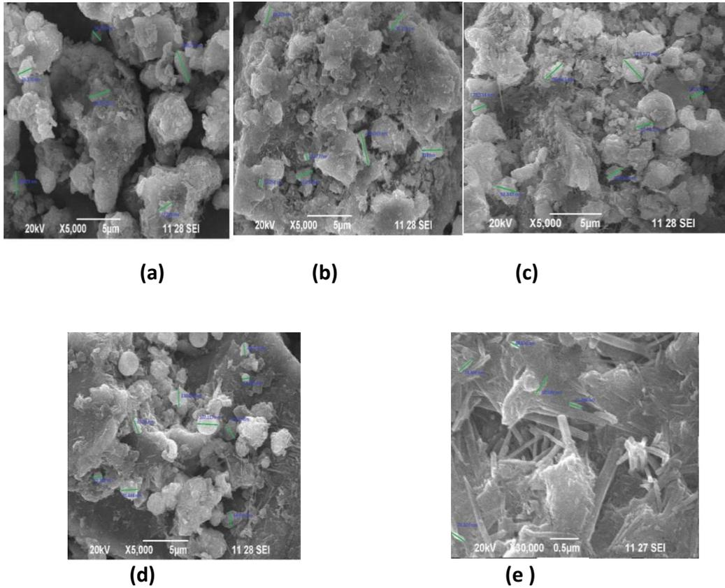
**Figure 7. SEM images of cement mortar on 28<sup>th</sup> day with NFA(a) 10% replacement of NFA (b) 20% replacement of NFA (c) 30% replacement of NFA (d) 40% replacement of NFA(e) 50% replacement of NFA**
