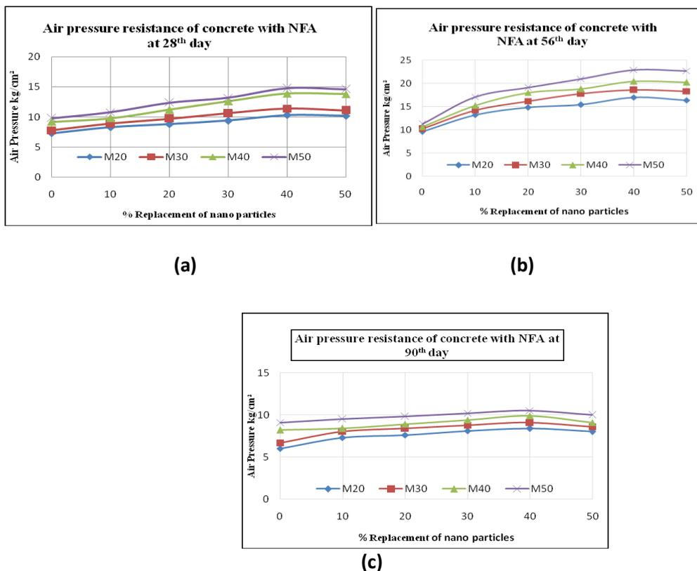
**Figure 11. Air pressure resistance of concrete NFA (a) Concrete at 28<sup>th</sup> day (b) Concrete at 56<sup>th</sup> day (c) Concrete at 90<sup>th</sup> day**
