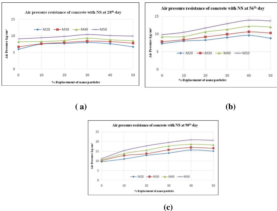
**Figure 12. Air pressure resistance of concrete with NS(a) Concrete at 28<sup>th</sup> day (b) Concrete at 56<sup>th</sup> day (c) Concrete at 90<sup>th</sup> day**
