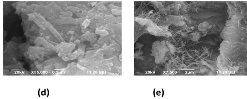
**Figure 8. SEM images of cement mortar on 28<sup>th</sup> day with NSF (a)10% replacement of NSF (b) 20% replacement of NSF (c) 30% replacement of NSF (d) 40% replacement of NSF(e) 50% replacement of NSF**
