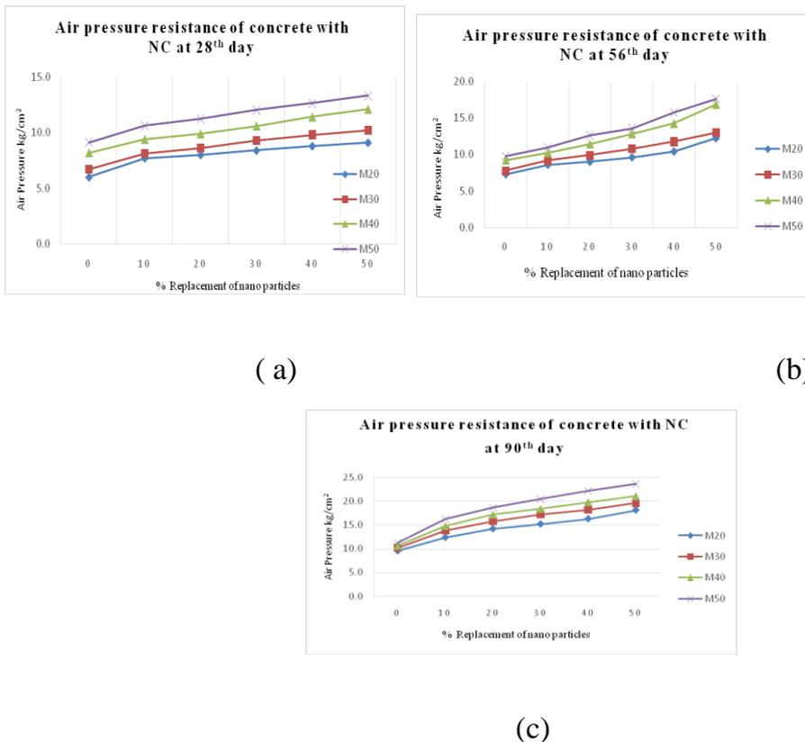
**Figure 10. Air pressure resistance of concrete with NC(a) Concrete at 28<sup>th</sup> day (b) Concrete at 56<sup>th</sup> day (c) Concrete at 90<sup>th</sup> day.**
