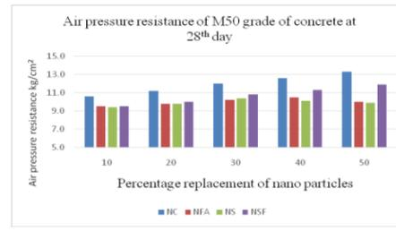
Figure 14. Air pressure resistance of concrete with nano particles at 28<sup>th</sup> day
