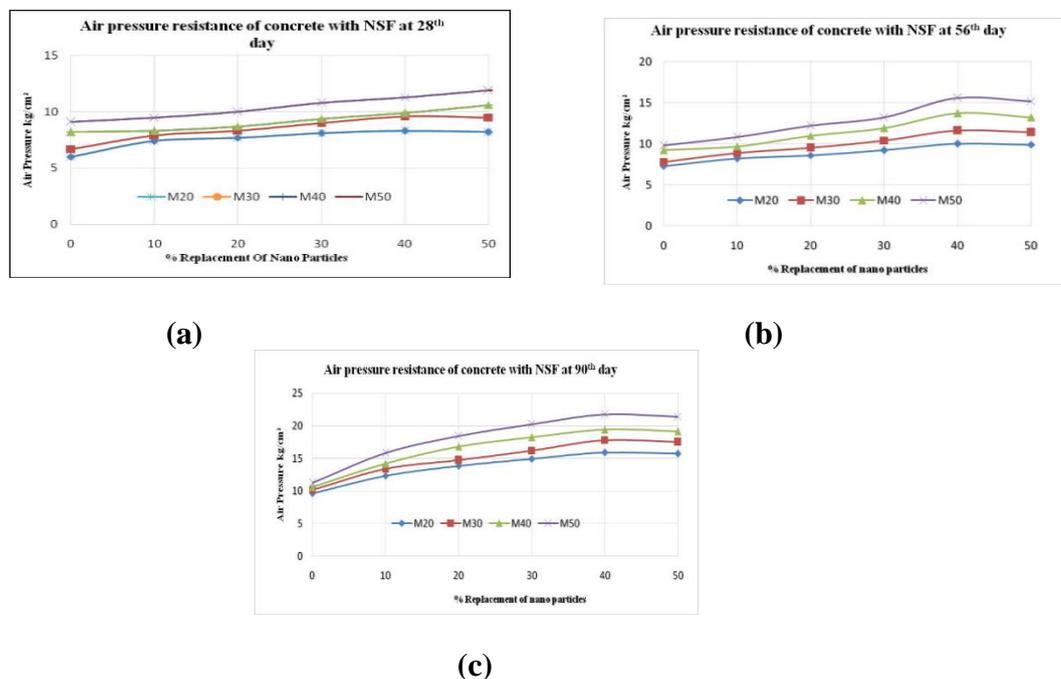
**Figure 13. Air pressure resistance of concrete with NSF (a) Concrete at 28<sup>th</sup> day (b) Concrete at 56<sup>th</sup> day (c) Concrete at 90<sup>th</sup> day**
