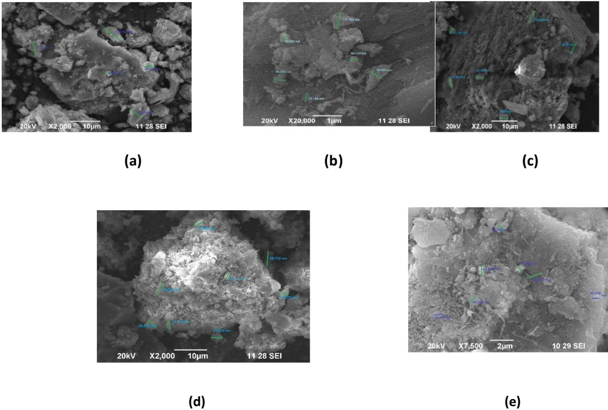
**Figure 6. SEM images of cement mortar on 28<sup>th</sup> day with NC(a) 10% replacement of NC (b) 20% replacement of NC (c) 30% replacement of NC (d) 40% replacement of NC (e) 50% replacement of NC**
