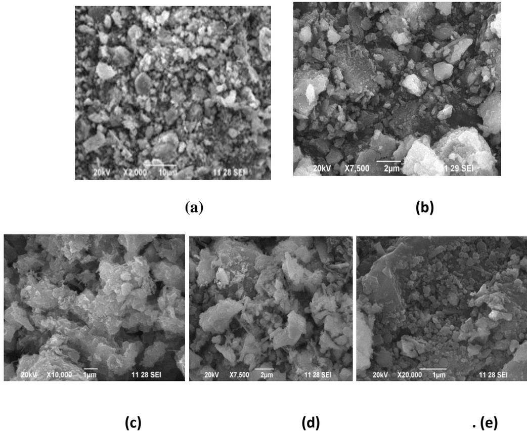
**Figure 9. SEM images of cement mortar on 28<sup>th</sup> day with NS(a)10% replacement of NS (b) 20% replacement of NS (c) 30% replacement of NS (d) 40% replacement of NS(e) 50% replacement of NS**
