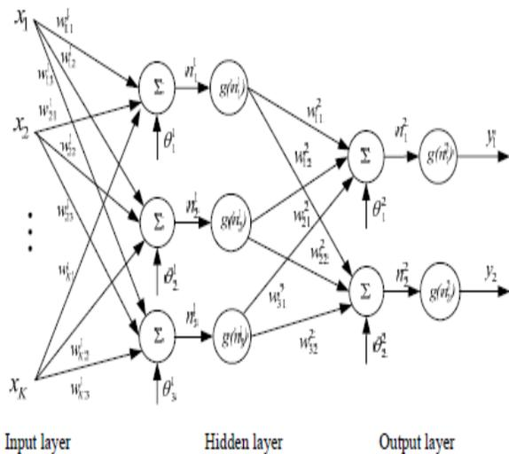
Fig. 5. A multilayer perceptron network with one hidden layer.
