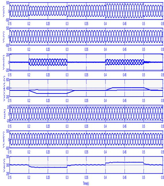
Fig. 7. Dynamic performance of DVR with in-phase injection during voltage sag and swell applied to critical load.
