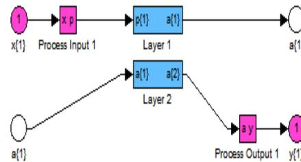
Fig. 6. Simulink structure of artificial neural network controller
