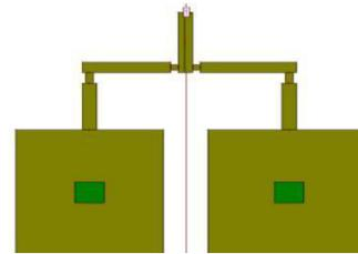
**Fig. 4: Weight machine square cut Shape Patch Antenna**
