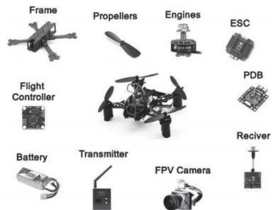
Fig: Basic components of Drone
