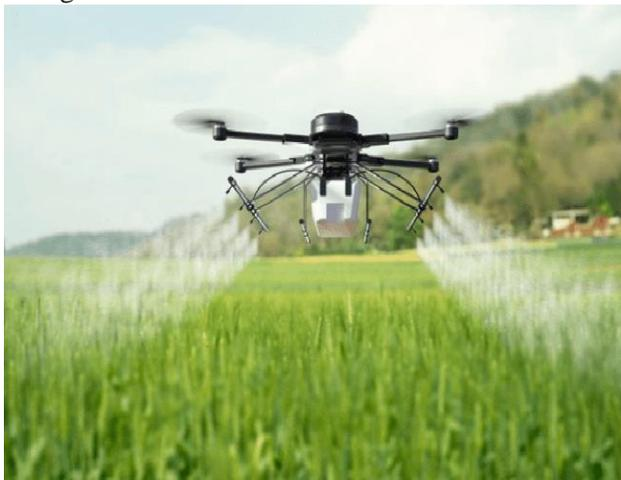
Fig: Drone Used For Spraying
