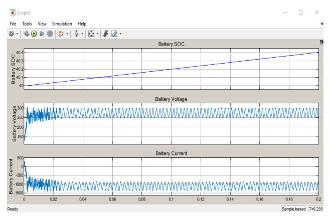
Fig 7 battery SOC, Battery voltage and battery current for EV3 Station
