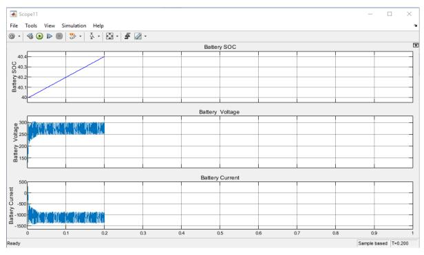
Fig 5 battery SOC, Battery voltage and battery current for EV1 Station
