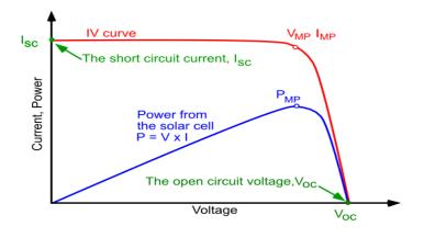
Figure 1: PV Panel Characteristic Curves
