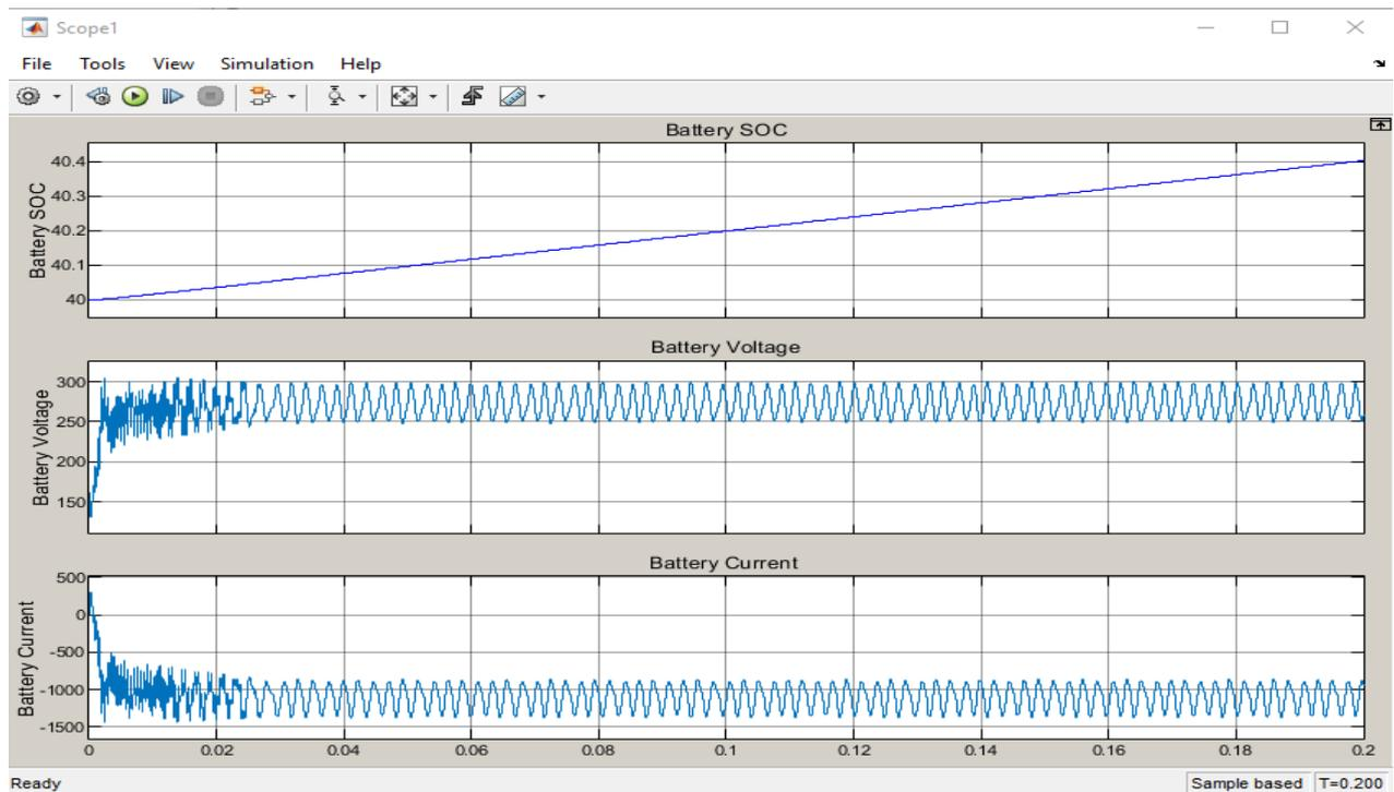
Fig 8 battery SOC, Battery voltage and battery current for EV2 Station
