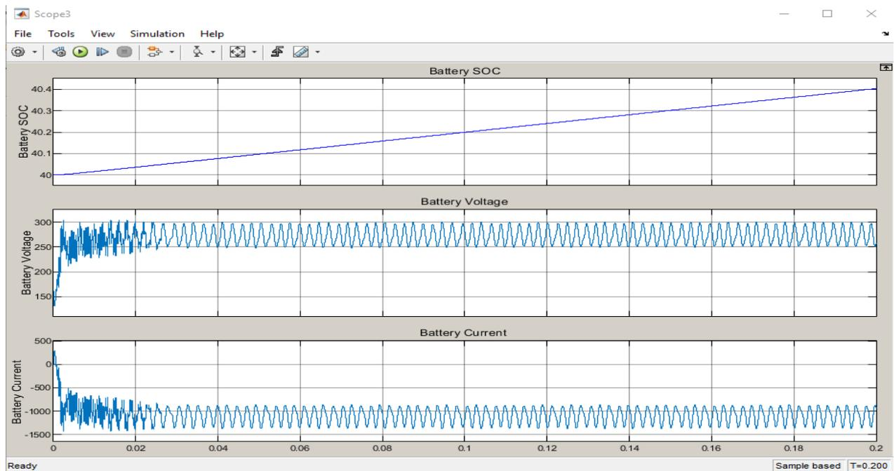
Fig 6 battery SOC, Battery voltage and battery current for EV4 Station
