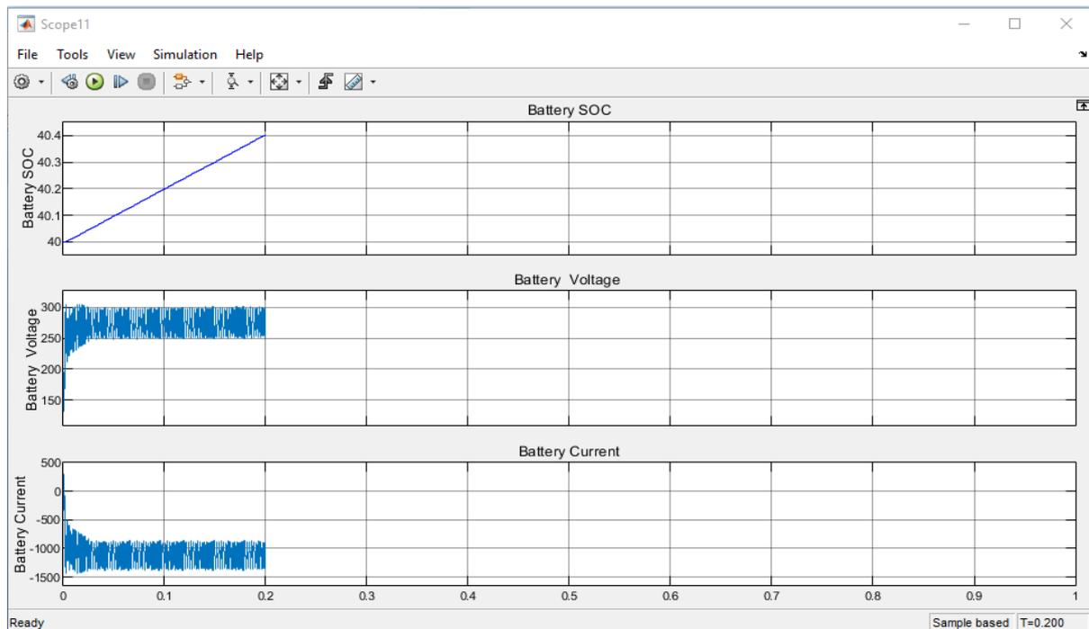
Fig 5 battery SOC, Battery voltage and battery current for EV1 Station
