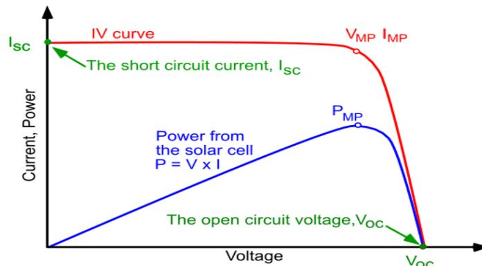
Figure 1: PV Panel Characteristic Curves
