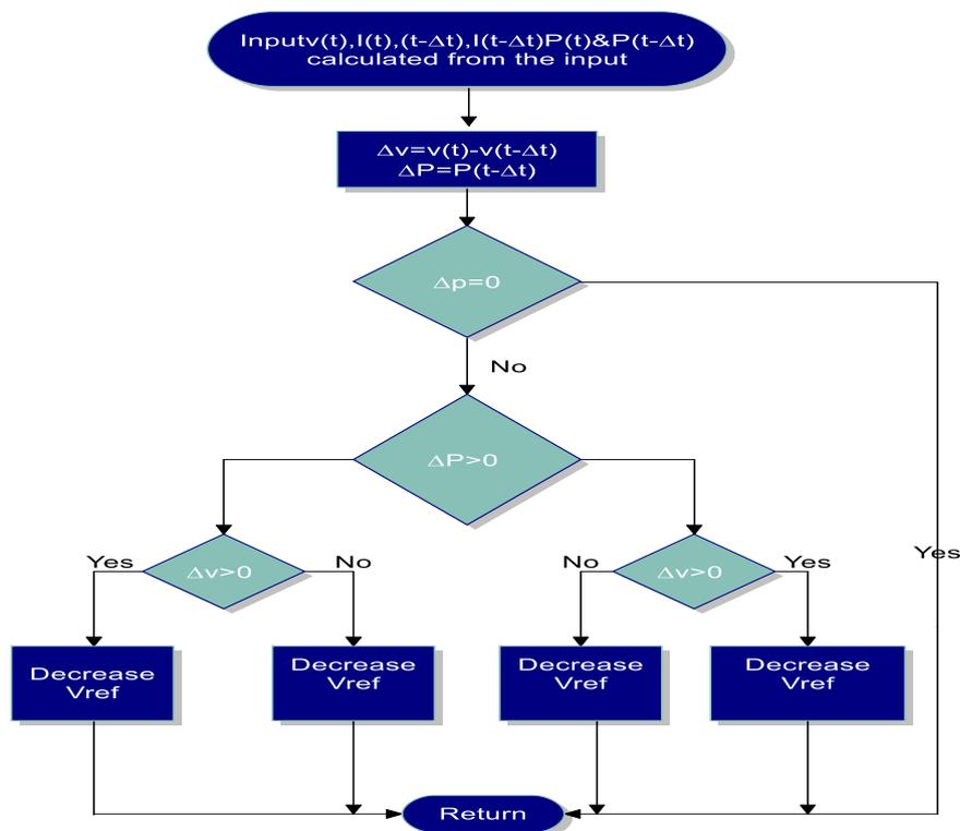
Figure 2: The Flowchart of the P&O Algorithm
