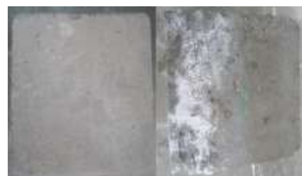
Fig. 3.3 - Sulphate Attack Test
