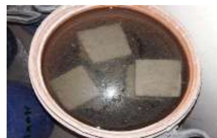
Fig. 3.2 - Cubes in Water Absorption
