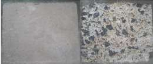
Fig. 3.5 - Acid Attack Test
