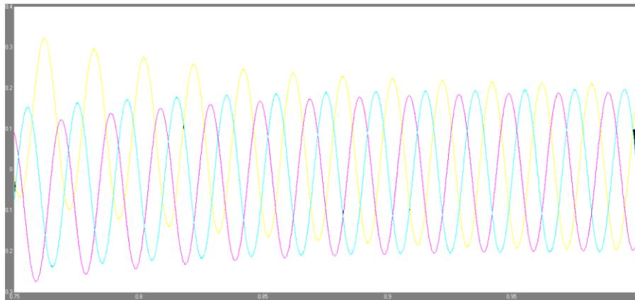
Figure 3. Graph When DVR is disconnected
