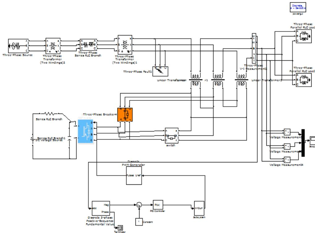
Figure 5. Simulation model of Dynamic Voltage Restorer
