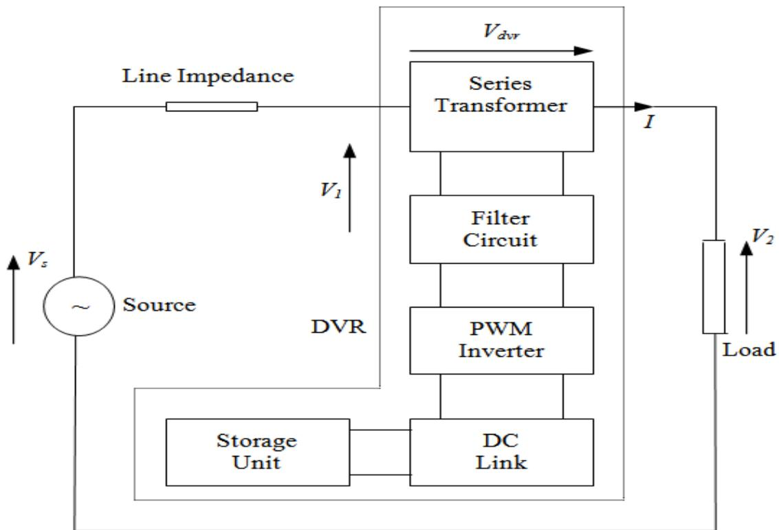
Figure 2. Block diagram of the DVR controller
