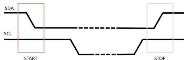
Figure 3 I2C Start and Stop Conditions in testing
