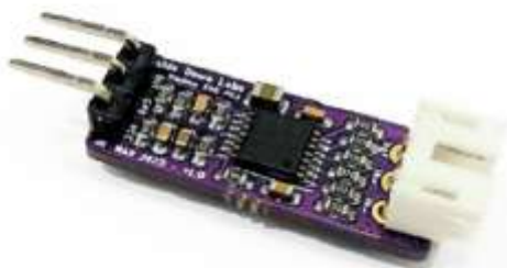
Figure 4.1.1: BIOAMP EXG Pill (EOG sensor)
