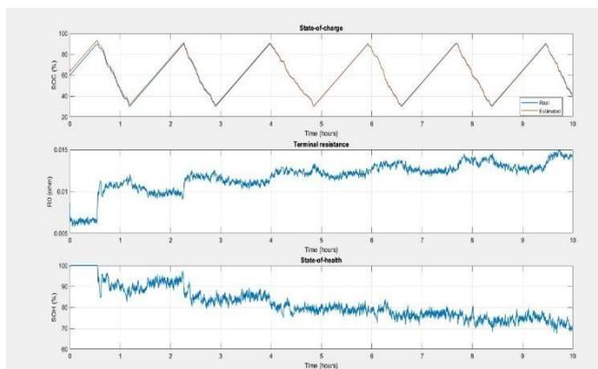
Fig 4. Graphical representation of Terminal Resistance, SOH, Time
