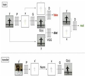
Normalization, on the other hand, is the process of scaling and centering the pose data to reduce the impact of variations in the lighting, background, and camera position. This helps to make the pose data more consistent and easier for the deep learning model to learn from. In the "Everybody Dance Now" project, the normalization step involves scaling the pose data to a fixed size and centering it at the origin.
