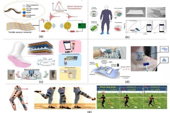
Fig 5. Wearable sensing systems include battery-free, self-sustainable nodes, textile-based smart wearables, and imperceptible energy harvesting patches [4].
