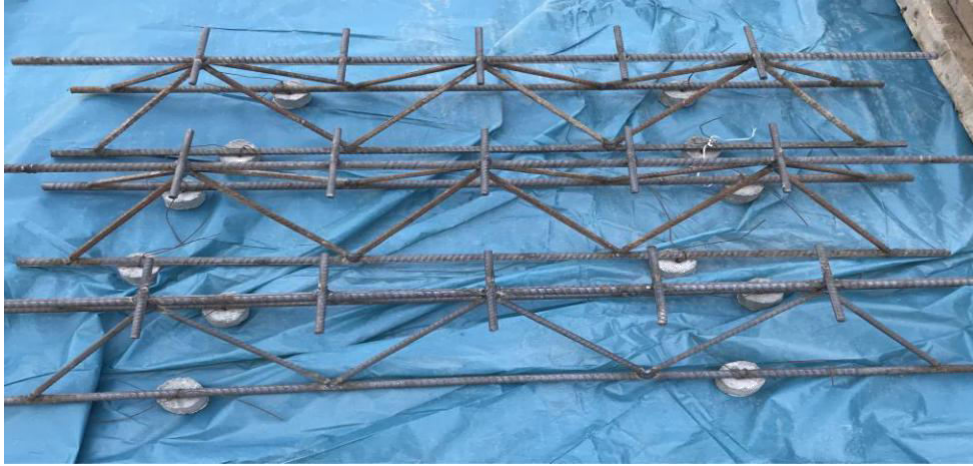
Fig No. 2 Lattice reinforcement
