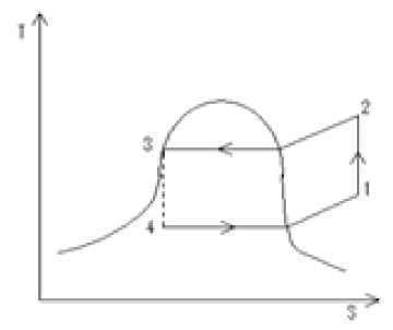
Fig.1: Temperature-entropy diagram of the cold room storage cycle processes
