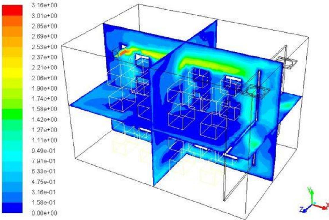
**Fig5 cold storage bucket with duct velocity in central plane**
