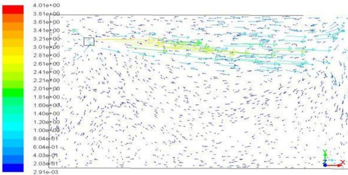
**Fig 6 cold storage velocity vector graph**
