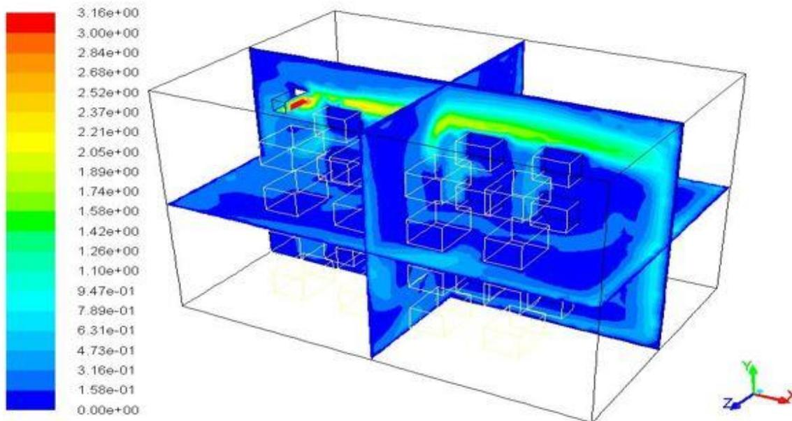
Fig 4 cold storage bucket velocity in central plane
