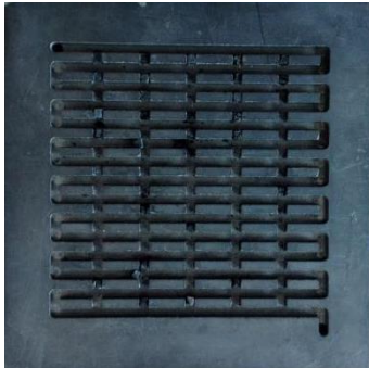
FIG 5.6 36 CM 2 SERPENTINE FLOW FIELD WITH 4 MM POROUS INSERTS - UNIFORM PATTERN
