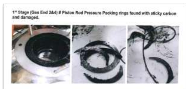
Fig 4 Damaged piston rings of the compressor during hot startup process
