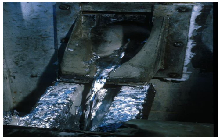
Figure – Cavity pouring of Material A356
