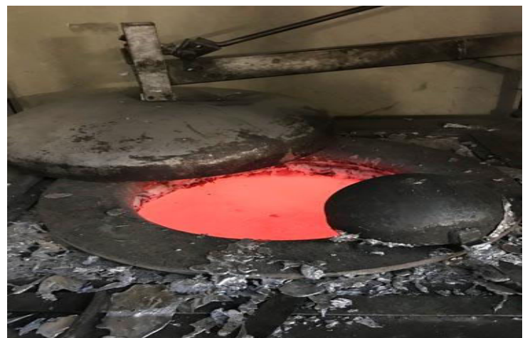
Figure - Temperature monitoring of squeeze die casting process with material A356
