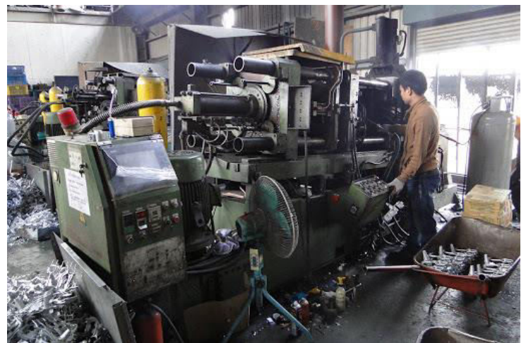
Figure - Temperature monitoring of squeeze die casting process with material A356
