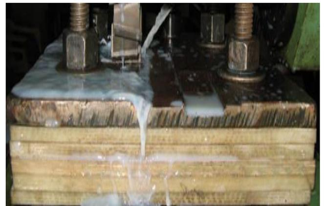
Fig 6.5. Five layers of Carbon fiber polyester bolted to the slotted table milling machine
