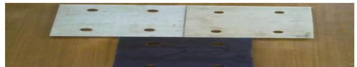
Fig . 6.1. Carbon fiber polyester, carbon fiber epoxy and mild steel plate.
