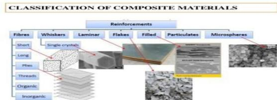
Fig.2.1 Classification of composite material
