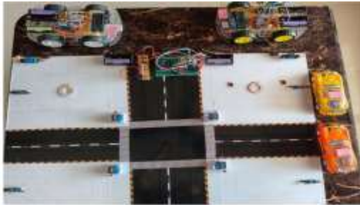
Fig 3 - Hardware Prototype of the Proposed Smart Parking and Wireless EV Charging System
