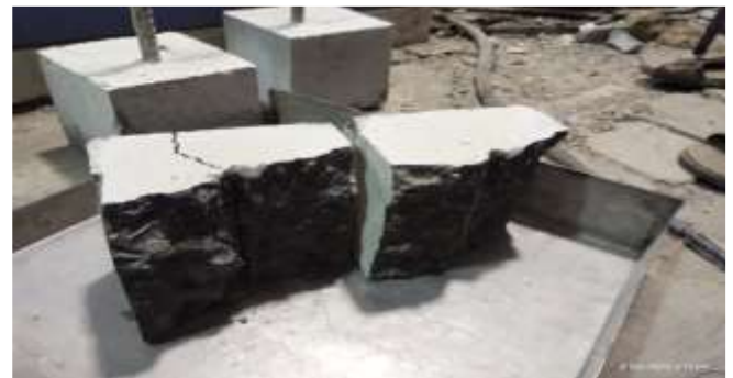
Fig 4.1 Pullout type of Failure
