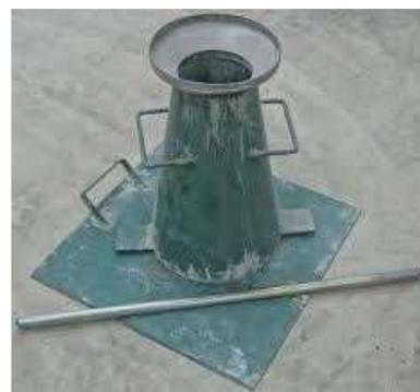
Fig. 4. Slump flow test
