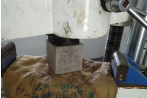
Fig. 6. Compressive Strength Test
