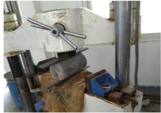
Fig. 7. Indirect Tensile Strength Test
