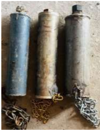
Fig-3 : Cylindrical PCM capsules fabricated from aluminum, cast iron, and stainless steel
