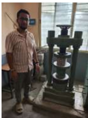
Fig 3.2.1 : Compressive strength testing
