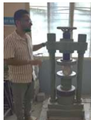
Fig 3.3.1 : Split tensile strength testing
