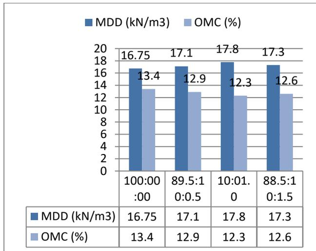
**Fig-1** Variations b/w MDD and OMC of Wheat Husk Ash, Sisal Fiber & soil with different proportions
