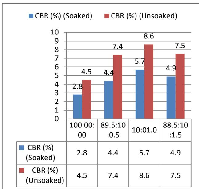
**Fig:-3** Variations b/w CBR Values of Clayey soil, Wheat Husk Ash and Sisal Fiber with different proportions
