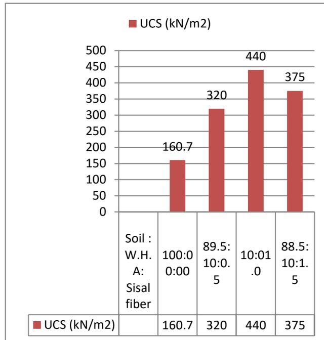
**Fig-2** Variations b/w UCS Values of Clayey soil, Wheat Husk Ash and Sisal Fiber with different proportions
