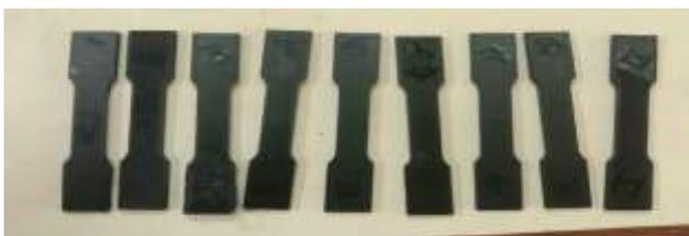
composite tensile bars with 9 different parameters
