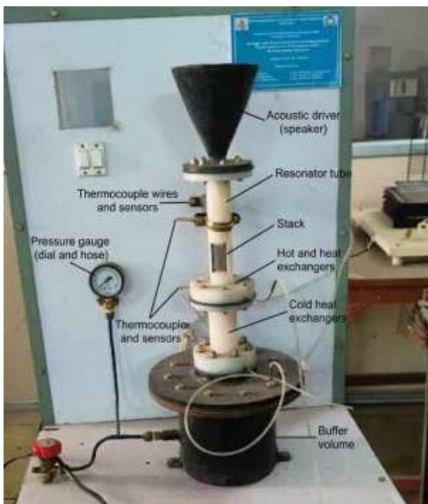
Fig -4: Experimental Setup of Thermoacoustic Refrigeration System
