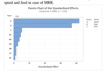
Figure 3 reveals the effect of speed, feed and DOC on the
