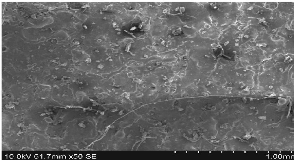
Fig. 6 – SEM images of surface using EDM process
