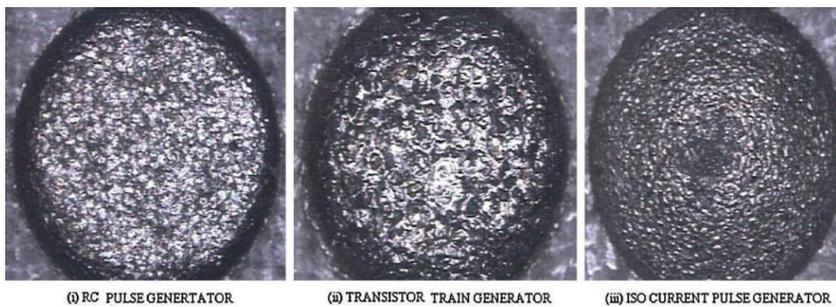
Fig. 5 – Surface topography of machined surface using different pulse generators.
