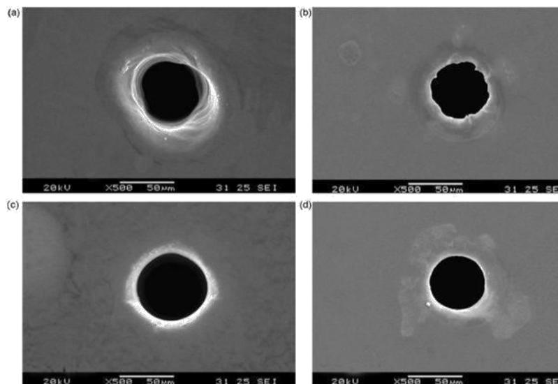
Fig,2 a) and (b) Hole entrance and exit drilled at 35V<sup>3</sup>, (c) and (d) Hole entrance and exit drilled at 30V<sup>3</sup>
