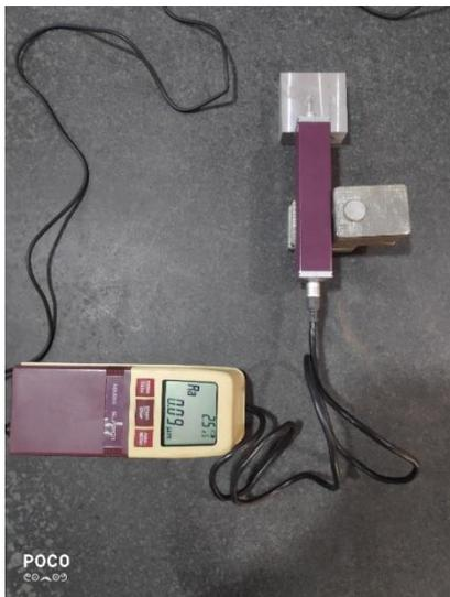
Figure 4 Surface Roughness Measurement
