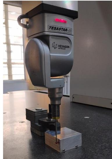
Figure 3 Perpendicularity measurement on CMM
