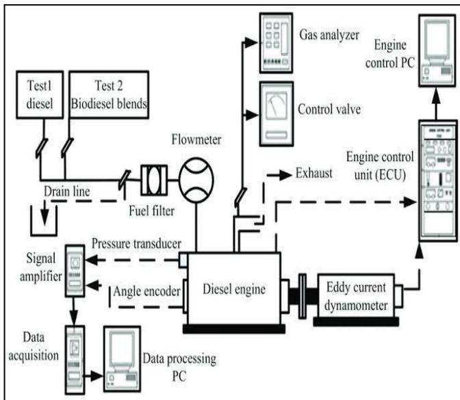
**Fig 4: EXPERIMENTAL ENGINE SET UP**
