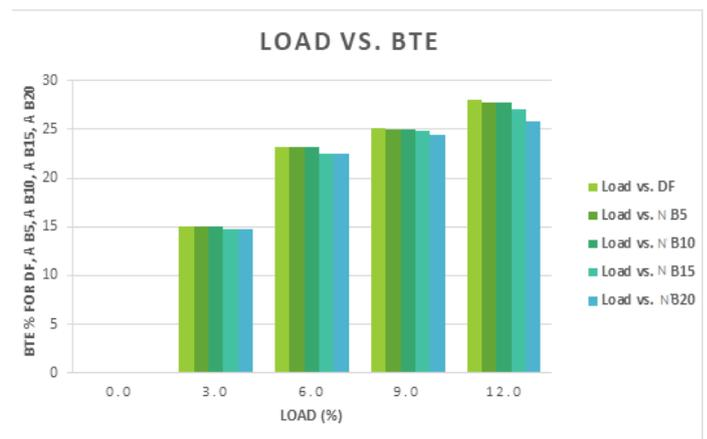
**FIG 5: Load vs Break Thermal Efficiency**
