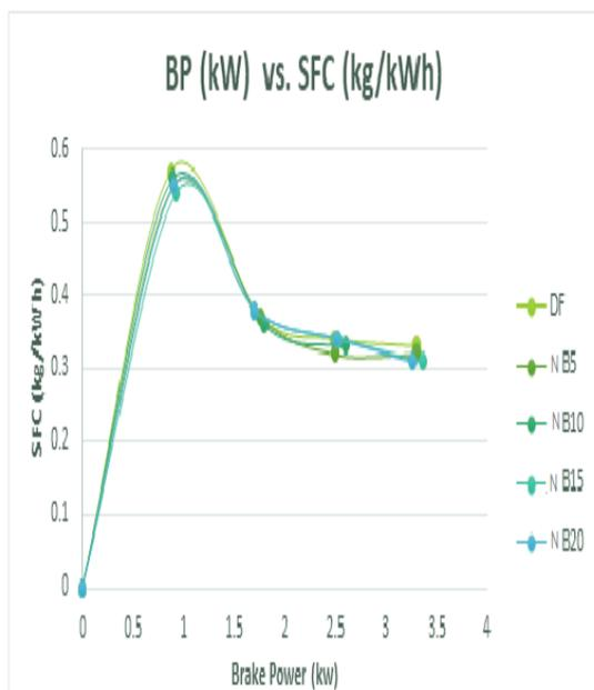
FIG 7: Break Power vs SFC
