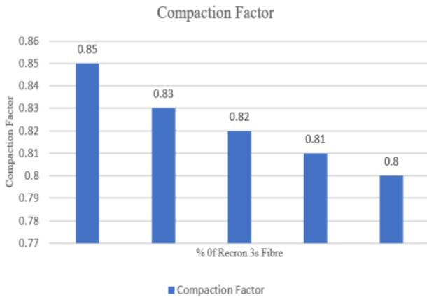
**Graph : Workability in terms of compaction factor test VEE-BEE TEST**
