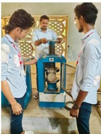
**Fig:** Split Tensile Strength
