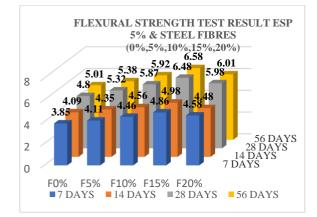
FIG.5.6: FLEXURAL STRENGTH BAR CHART TEST
