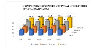
FIG.: 5.2 COMPRESSIVE STRENGTH BAR CHART @ ESP 5% & STEEL FIBRES (0%,5%,10%,15%,20%)
