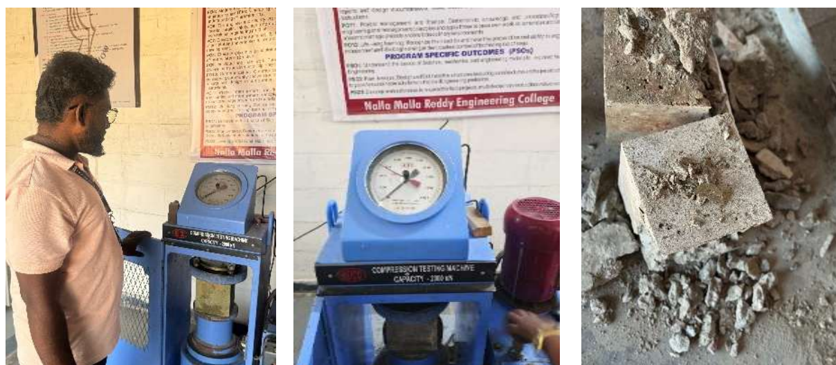
Figure 3: Performing the compressive strength test
