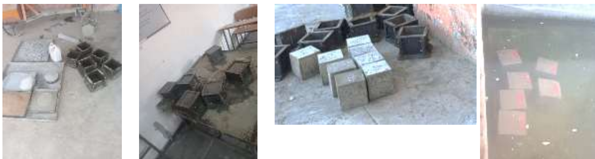
Figure 2: Concrete specimen preparation, casting, demoulding, and curing
