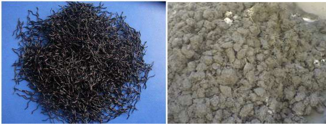
Figure 3.1 Round Crimped Steel fibre Figure 3.2 Mixing of fibres in concrete
