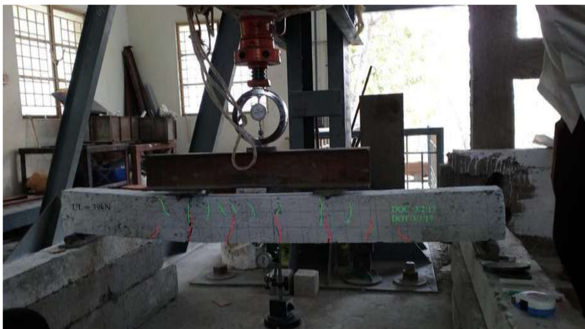
Figure 4.4 Failure of the SFRC beam
