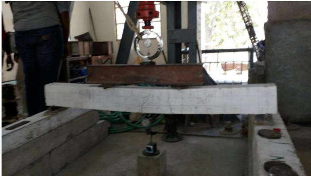
Figure 3.3 Experimental setup for flexural members
