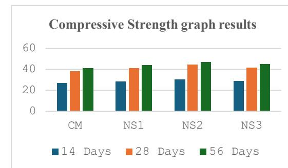
The results show that nano-silica significantly improves compressive strength at all curing ages. Maximum strength was observed at 2% nano-silica replacement. The improvement is attributed to accelerated hydration and densification of the cement matrix.
