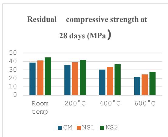
Strength decreased with increase in temperature for all mixes. However, nano-silica blended concrete consistently retained higher residual strength. The NS2 mix exhibited the highest strength retention at all temperature levels.
