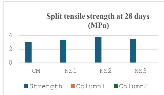
Nano-silica improved split tensile strength due to refinement of the interfacial transition zone and reduced crack propagation.
