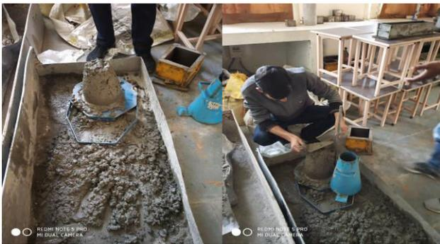
**Fig .1 Slump testing by Slump cone apparatus with different percentages of plastic**
