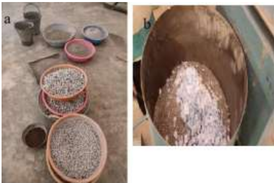
Fig. 10: Prepared ingredients and mask pieces used during concrete mixing
