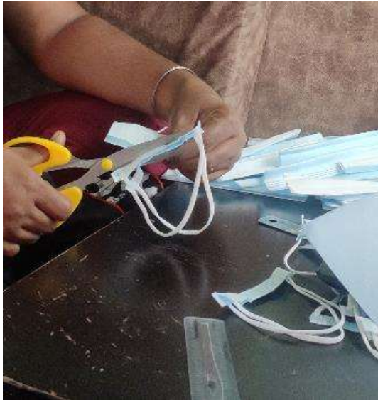
Fig. 4: Cutting of discarded face masks into reinforcement pieces
