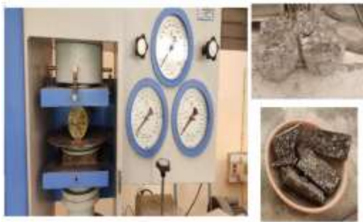
Fig. 8: Split tensile strength test and broken specimens
