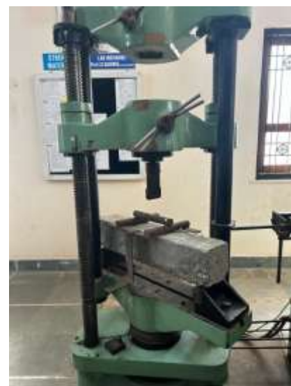
Fig. 3.7 : Flexural Strength Testing
