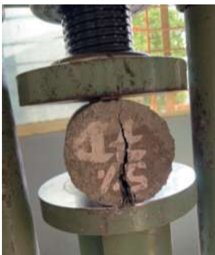
Fig. 3.5 : Split Tensile Strength Testing
