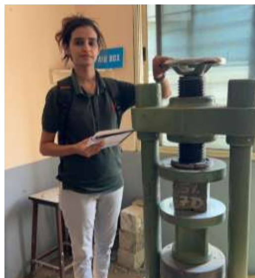
Fig. 3.3 : Compressive Strength Testing
