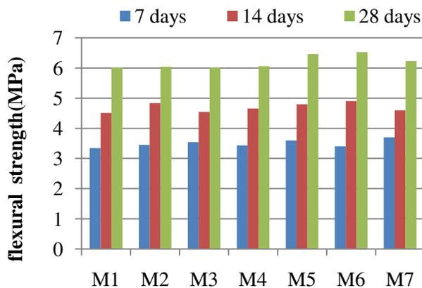
Fig. 4 Comparison of flexural strength for different mixes
