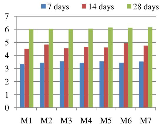
Fig. 3 Comparison of split tensile strength for different mixes
