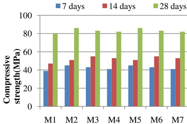
Fig. 2 Comparison of compressive strength for different mixes
