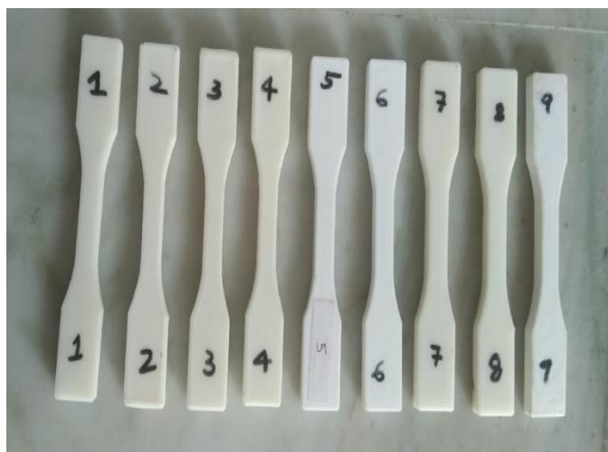
Figure 4.1: 3D printed Tensile specimens
