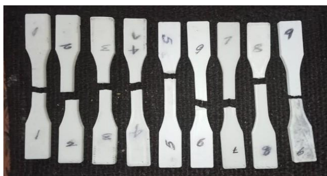
Figure 4.2: Tensile specimens after testing
