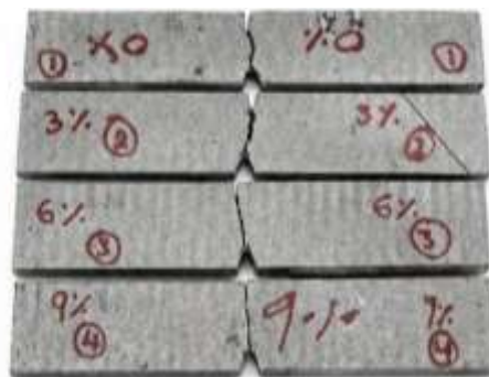
Figure 3.3 Impact fractured specimens 0%, 3%, 6% and 9% composites
