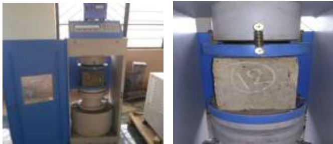
Fig 3.2.1 : Compressive strength testing
