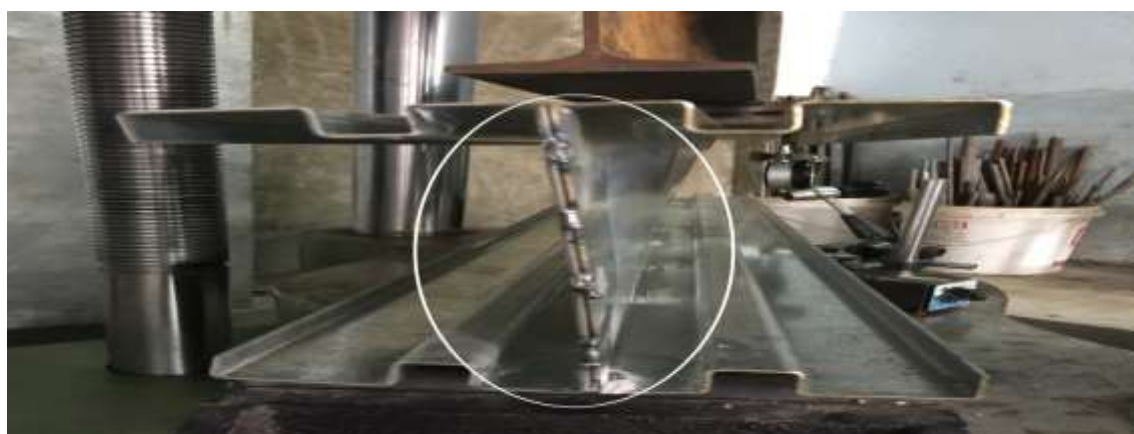
Fig 4 Lateral torsional buckling in web of cold formed I section without intermediate stiffener
