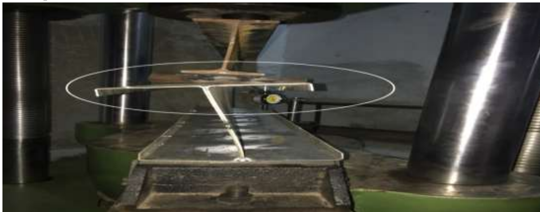
Fig 3 Distortional buckling of compression flange of cold formed I section without intermediate stiffener
