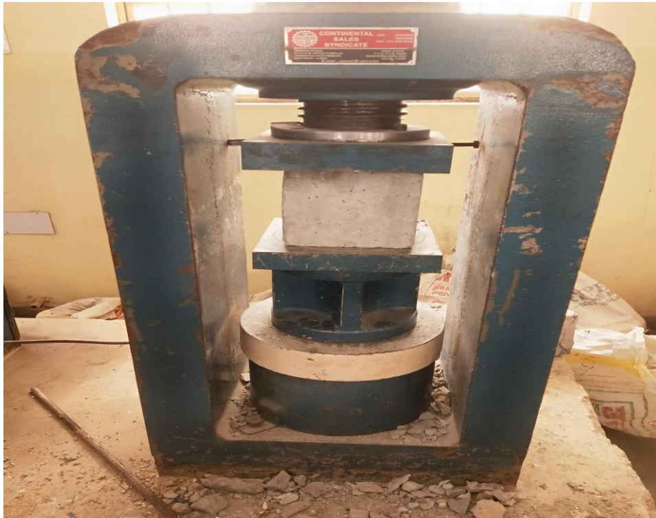
Fig. 2 Compressive test of cube
