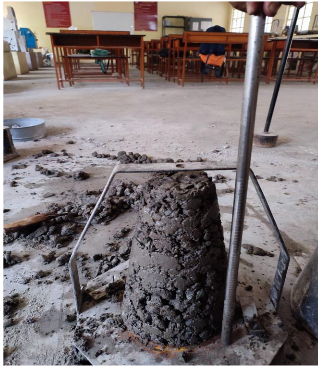
Fig. 3: Slump of Concrete at 60% Replacement
