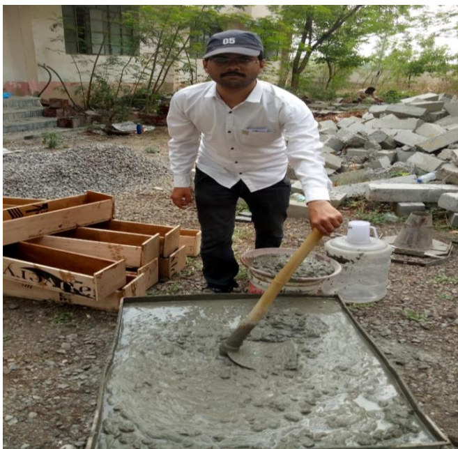
Fig. -1 Over burnt brick bats added to concrete
