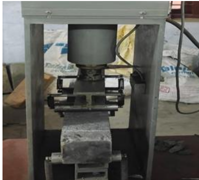
Fig -4: a) Bar diagram showing variation in split tensile strength b) Split tensile test
