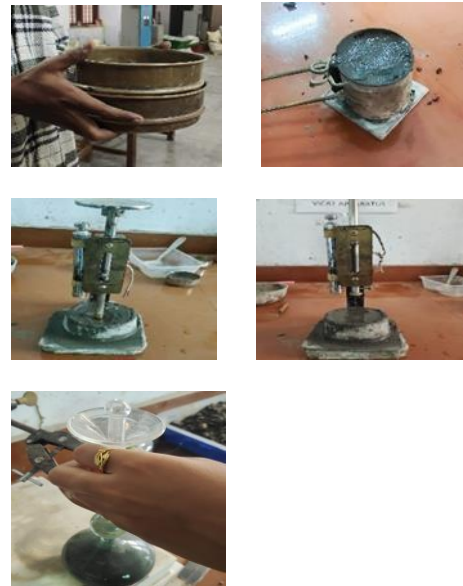
Fig -1: a) fineness, b) soundness c) consistency d) initial setting time e) specific gravity
