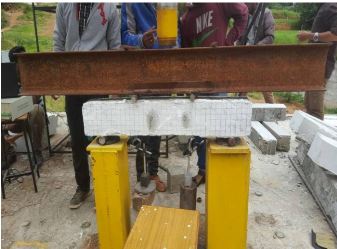
FIG1. TEST SET UP OF BEAM IN LOAD
